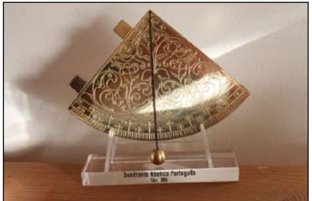
Figure 1. Portuguese Mariners Quadrant (Quarter of a Circle) showing sighting pin holes and plumb line.
