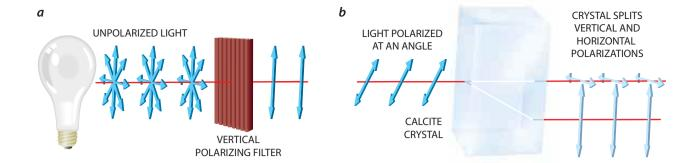
**UNPOLARIZED LIGHT** consists of photons that are polarized in all directions (*a*). In polarized light the photons' electric-field oscillations (*arrows*) are all aligned. A calcite crystal (*b*) splits a light beam in two, sending photons that are polarized parallel with its axis into one beam and those that are perpendicular
