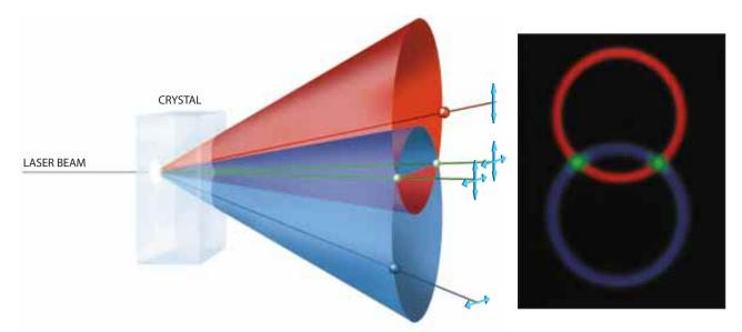
**ENTANGLED PHOTON PAIRS** are created when a laser beam passes through a crystal such as beta barium borate. The crystal occasionally converts a single ultraviolet photon into two photons of lower energy, one polarized vertically (*on red cone*), one polarized horizontally (*on blue cone*). If the photons hap-
